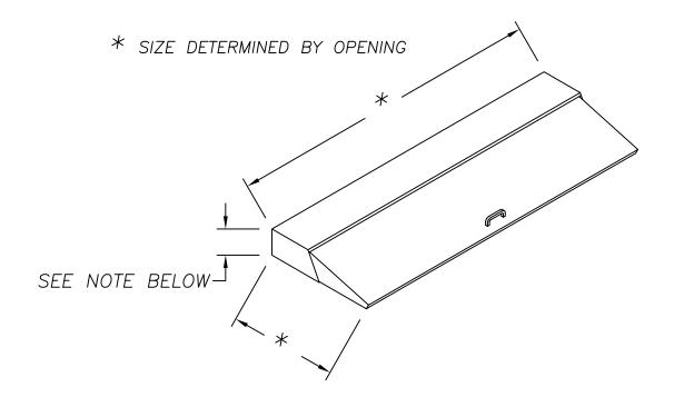
NOTE: FOR FRONT TO BACK DIMENSIONS OF 12" OR LESS, THE HEIGHT WILL BE 5 3/4", AND FOR OPENINGS GREATER THAN 12", THE HEIGHT WILL BE 10".
